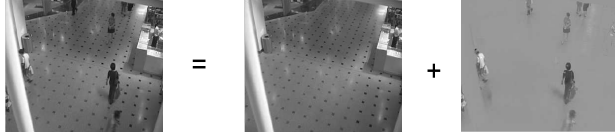
Figure 1: RobustXRAY applied to video background-foreground separation problem
